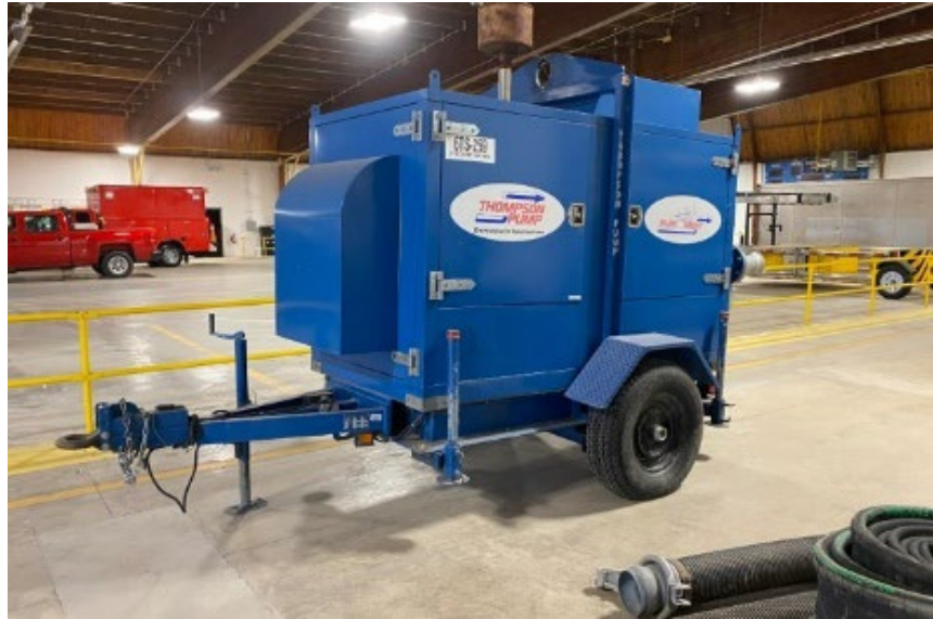
Portable Pump for deployment during flooding events
