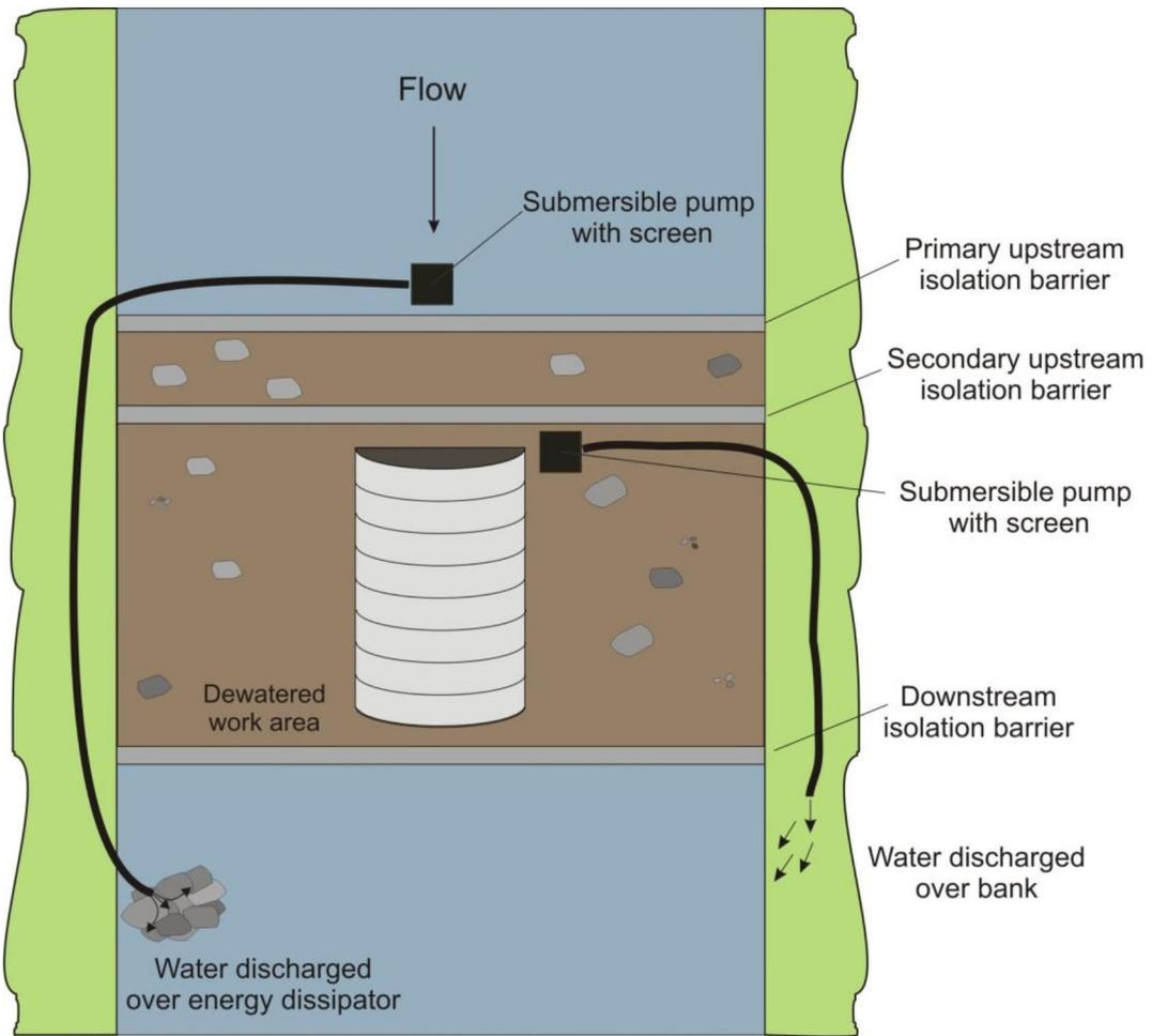
**Figure 3. Isolation and Bypass Diversion when Working In-Water**
