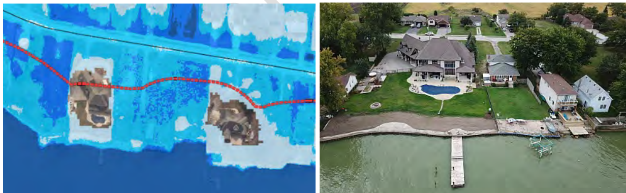
Figure 5.1 New Homes Properly Flood Proofed and at-risk Older Development (left mapping of the Flood Hazard Limit and right oblique photo)
